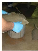
6. Strike-Off by Covering 2/3 and Sawing off the Surface. Then 2/3 Pushing Away.
