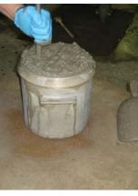
5. Measure must not Contain Substantial Excess or Deficiency of Concrete
